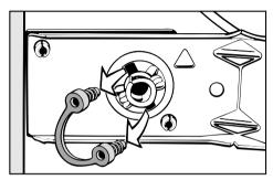
Using combination pliers, pull out the retaining clips on the right and left of the support plate.
